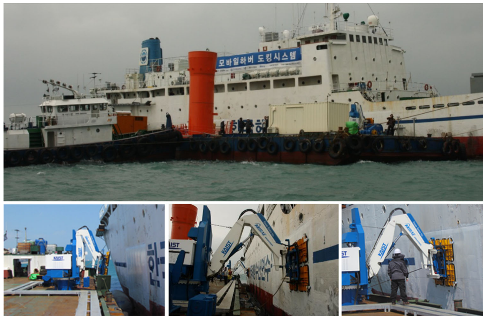
Fig. 14 Open-water ocean demonstration of the ship-to-ship automatic docking system from a barge
