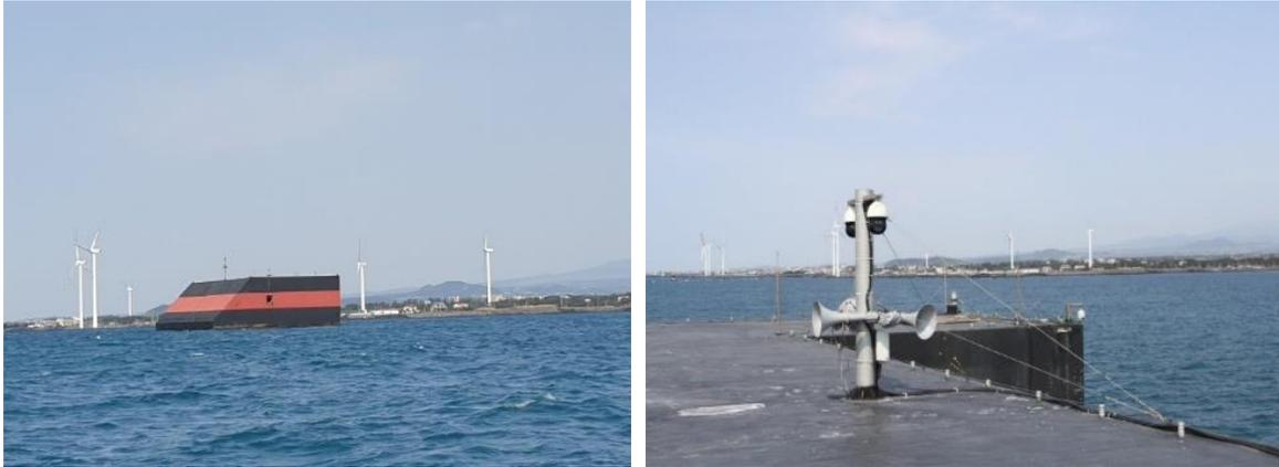
**Fig. 5.2.** Fixed-type wave energy converter installed at Jeju Island and CCTV camera.
