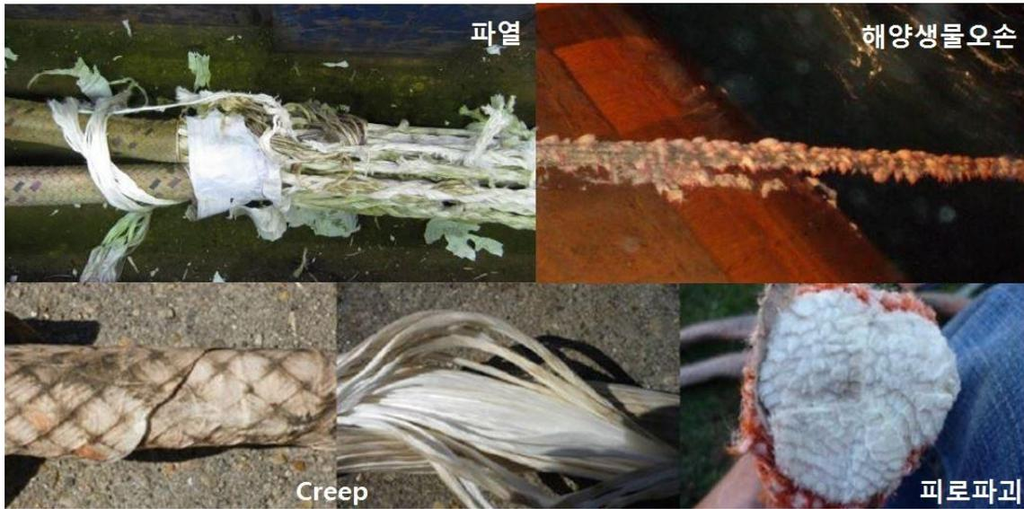
**Figure 4-17 Failure of cable in ocean environment**
