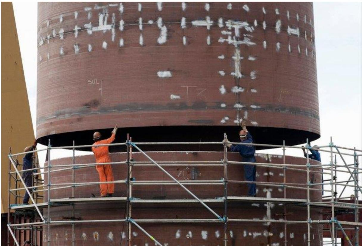
**Figure 4-13 Platform manufacturing by welding in WindFloat project**
