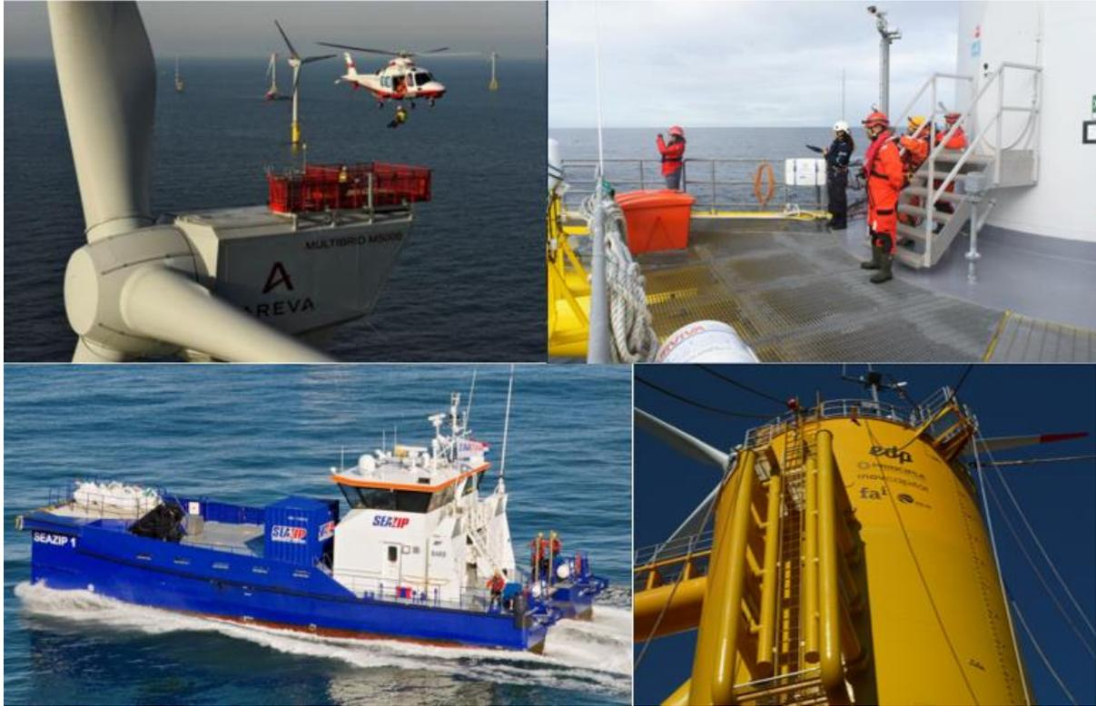
Figure 6-7 Ways to approach wind turbine
